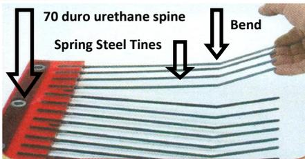
Wagner's brushes are made from our special High Performance Urethane. "Memorized" Spring Steel Tines are designed to snap back to its original position. The 70 durometer spine is designed to absorb shock and mitigate jam-ups. Best of all, our brushes outlive fiberglass brushes by many years. They are made for all corrugator models. Tips should never touch board.
