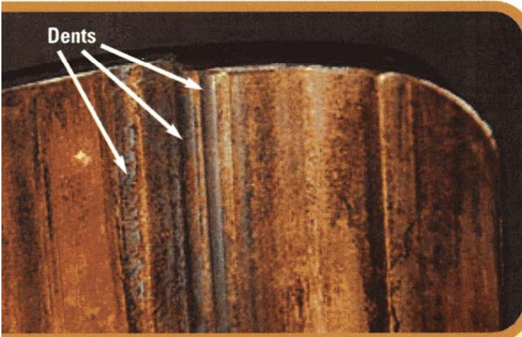
▲ Roller Dents on Old Design Jaw
