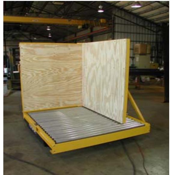
SCISSORS LIFT LOWERED WITH ADJUSTABLE BACK STOP.
